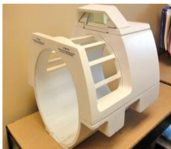
FIG (3): BIRDCAGE COILS
